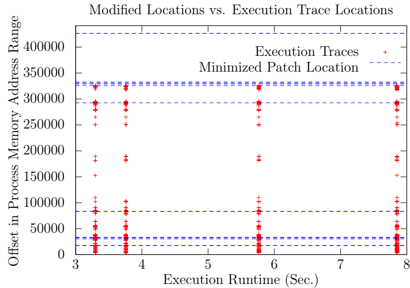
Figure 6.6: Fixes occur in different locations from execution traces: The location of every edit in a minimized successful repair is plotted as a horizontal line. Each vertical column shows points of execution traces from one test suite. Test suites shown from left to right are 3 tests (exploit tests only), 4, 7, and 11 tests (exploit and author-generated regression tests), with 330, 399, 518, and 596 sampled execution locations respectively. Code modifications occur in different locations from execution traces
